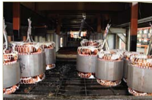
Automatic Impregnation Plant
